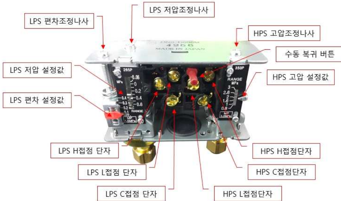
압력스위치 (Dual Pressure Switch, DPS)
